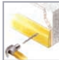
Fixing skirtings, rails and trims to blocks through plasterboard or insulation.
