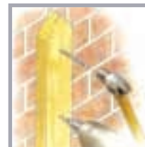
Fixing fence and gate posts to masonry.
