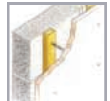
Fixing battens and timber frames to walls and floors for insulated linings and suspended floors.
