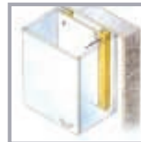
Fixing battens to blocks to support kitchen cupboards.
