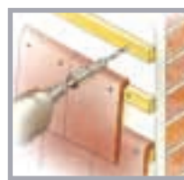
Fixing battens to bricks or blocks to support vertical tiling.
