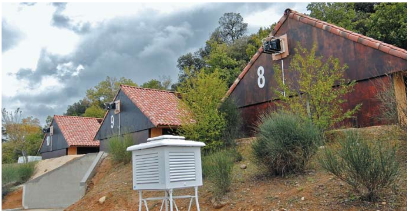
Example of ACTIS in-situ test cells, Limoux, France.
