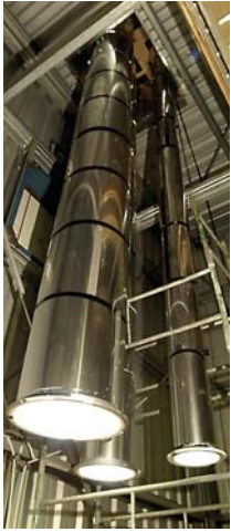
Internal view of different diameter tubular rooflights under test
