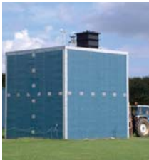
Monitoring of three tubular rooflights simultaneously
