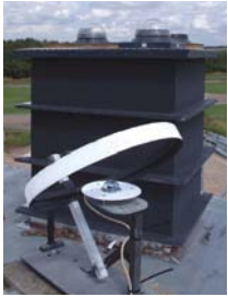
External lux sensor with shade ring for measuring diffused light levels
