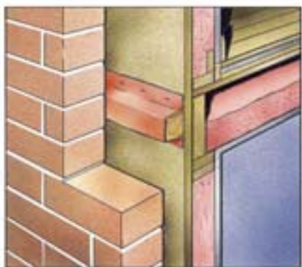
For separating floor junctions and eaves level
